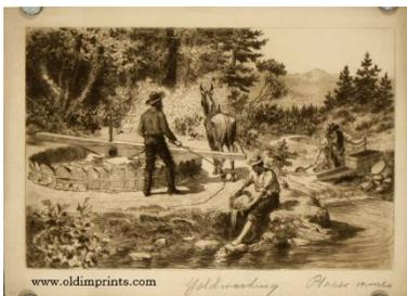
For gold ore, the gold was typically recovered by amalgamation with quicksilver. The miner would add clean mercury to the ground ore, continue grinding, rinse out the fines, then add more ore and repeat the process. At cleanup, the gold amalgam was carefully recovered from the low places and crevices in the arrastra floor. The
